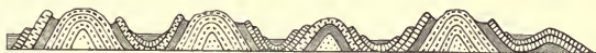
FIG. 134.—Section of the Jura Mountains, showing ridges following the anticlines and valleys along the synclines.
